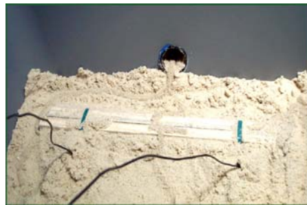
Foraging shelter tubes (in red in the left photo) are directed toward the electrical source in a laboratory test unit (middle photo). Far right C. formosanus soldier.
