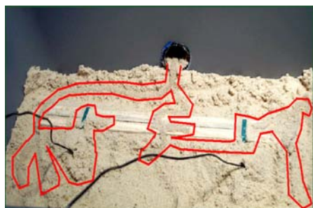
Foraging shelter tubes (in red in the left photo) are directed toward the electrical source in a laboratory test unit (middle photo). Far right C. formosanus soldier.
