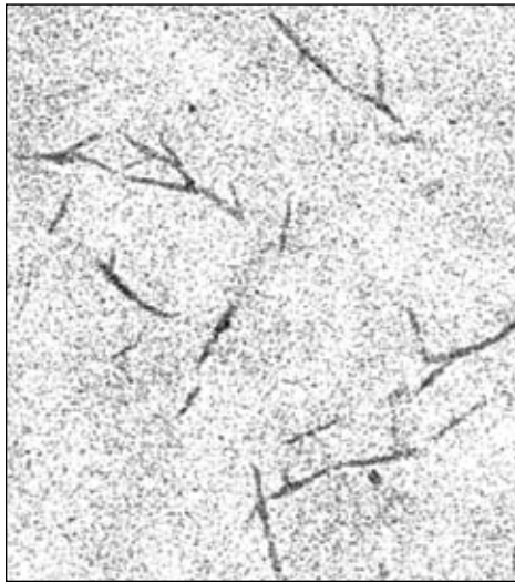
Micrograph of cellulose nanocrystals.
