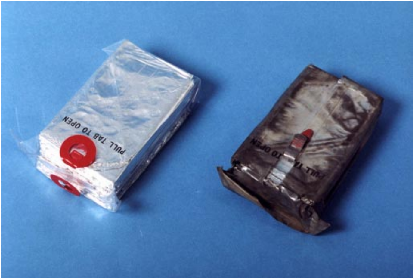
Figure 24—Frequent inspection keeps damaged shelters off the fireline.
