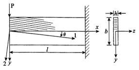
FIG. 1. Orthotropic cantiever subjected to single load. *x* and *y* are geometrical axes; 1 and 2 are material axes.
