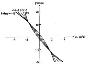
Fig. 3. Normal stresses  $(\mathbf{s}_*)$  at fixed end (x = 80 mm) for several grain slope values (**q**).
