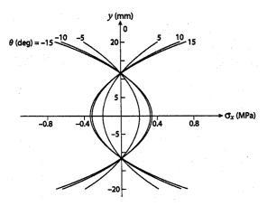
FIG. 2. Normal stresses  $(\mathbf{s}_x)$  at free end (x = 0 mm) for several grain slope values (q).
