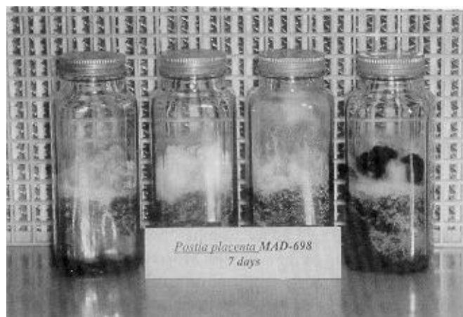
Fig. 1. Soil-block bottles showing 7-day cotton cellulose testing of P. placenta MAD-698. (Cellulose treatments left to right: ABTS; Control; \text{CeCl}_3 ; RR.)
