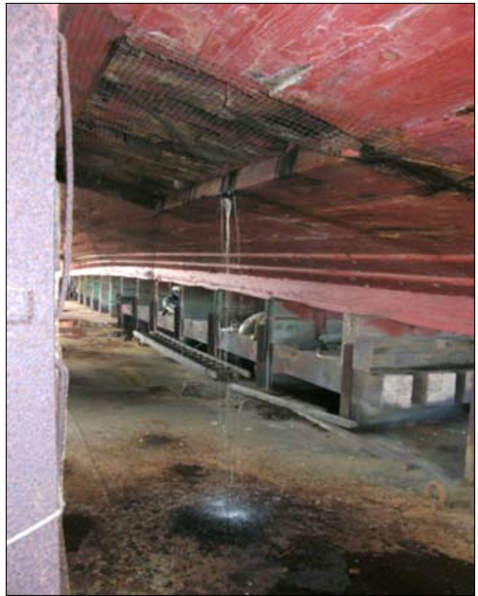
Hull planks removed to vent cargo hold (note rainwater seepage)
