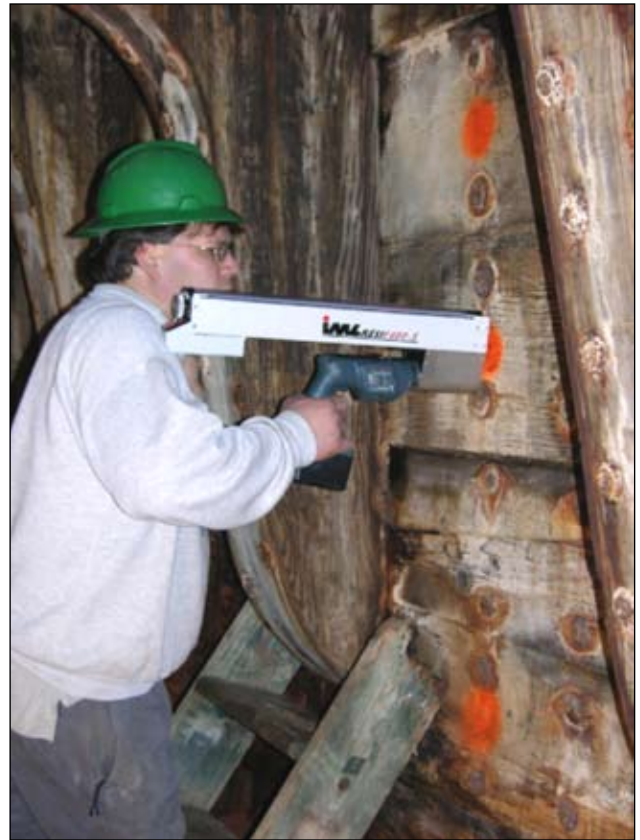
Resistance micro-drilling a clamp member
