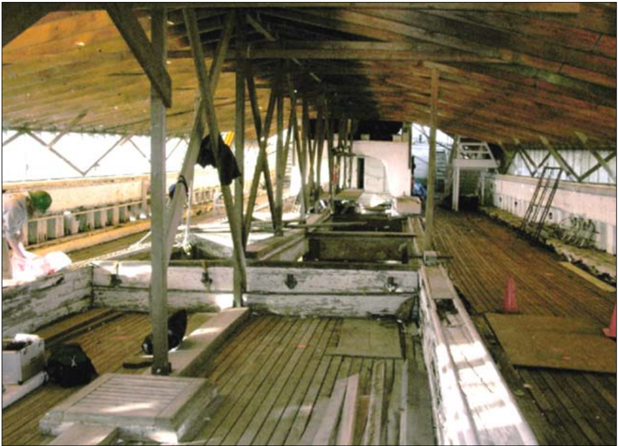
Aft view of main deck area showing main cargo hatch and overhead roof structure
