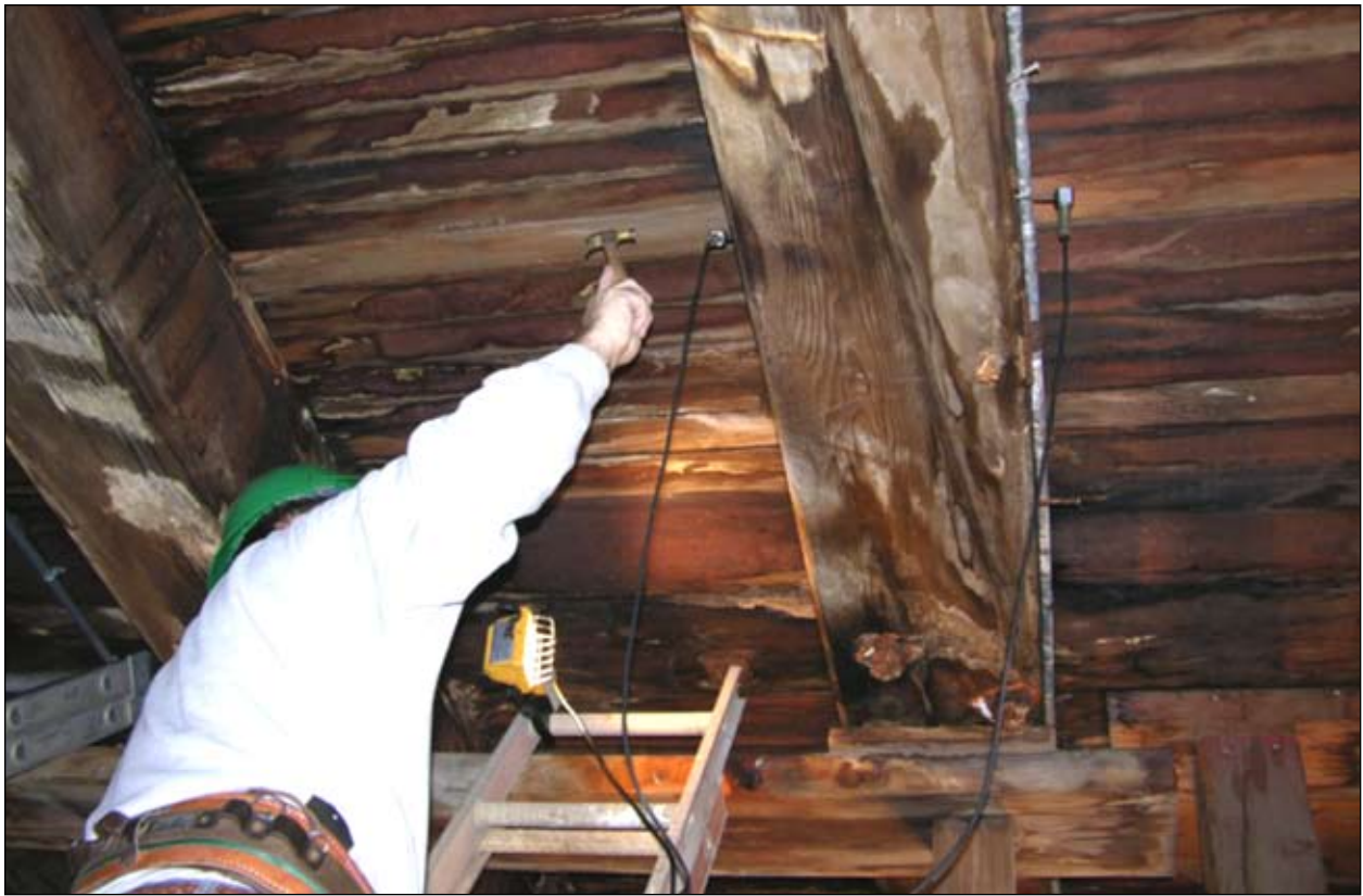
Stress wave timing measurements at main deck beam
