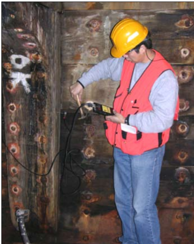
Stress wave timing measurements at hanging knee
