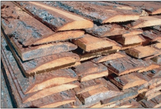
Figure 12—Example of slabs accumulated at sawmills.
