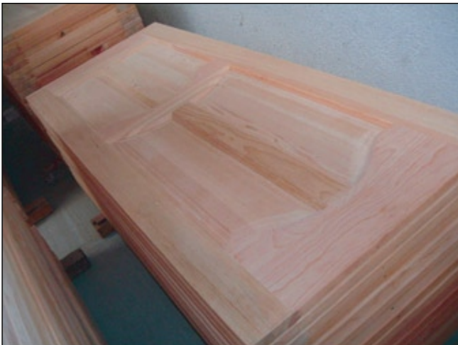
Figure 20—Floating-panel, solid-wood doors manufactured in Oaxaca.
