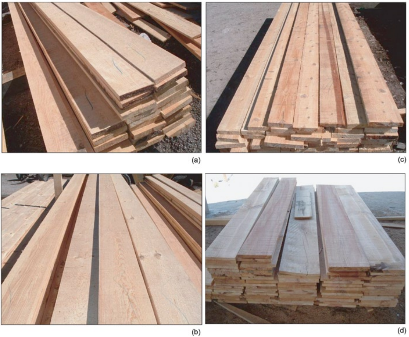
Figure 17—Representative boards from lumber grades: (a) “Firsts”: combination of No. 1 and No. 2 grade lumber; (b) No. 3 grade; (c) No. 4 grade; (d) No. 5 grade. See Table 2 for description of grades.
