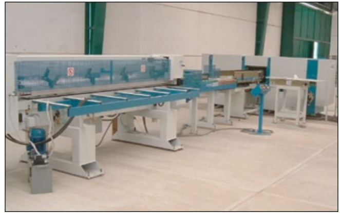
Figure 21—Modern finger-jointing system.
