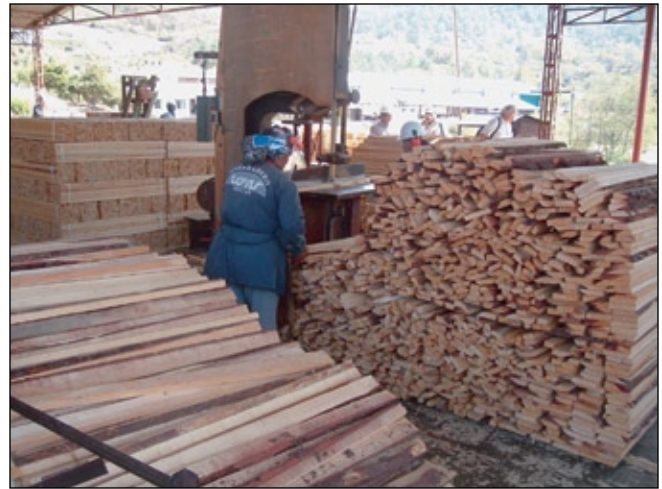
Figure 15—Lumber recovered from slabs is sawn into slats, pallet stock, and blanks for broom handles.
