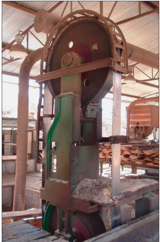
Figure 10—Large band saw used at sawmills.
