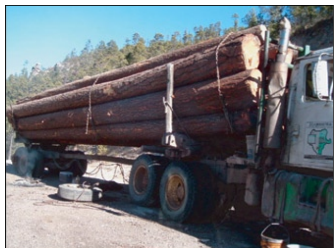
Figure 2—Specialized log-hauling semi-truck and trailer for carrying logs up to 24 ft (7.3 m) long.
