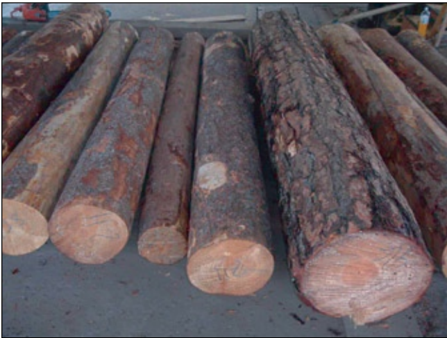
Figure 8—Mixture of species and diameters of logs queued for sawing. Large-diameter log on right with heavy bark structure is Pinus pseudostrobus ; other logs are P. patula .
