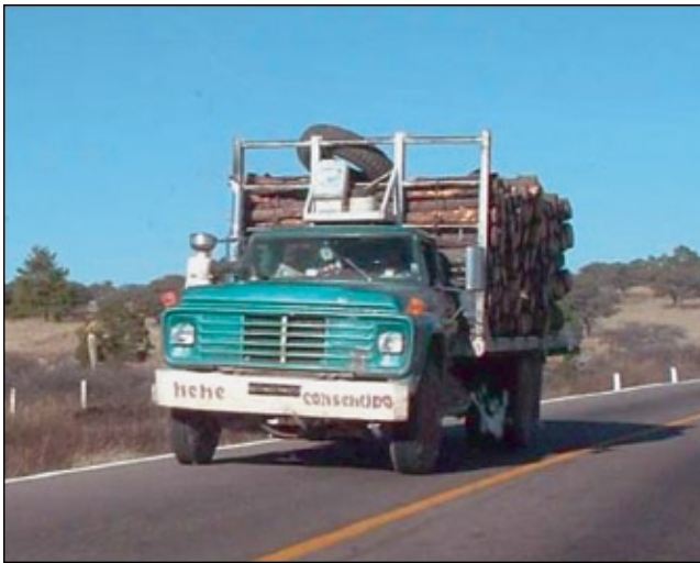
Figure 3—Typical heavy-duty truck for transporting logs cut to nominal length of 8 ft (2.4 m).
