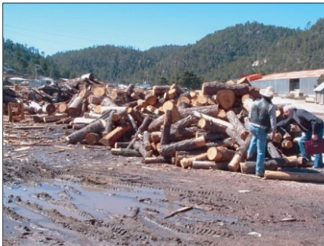
Figure 14—Large quantity of log shorts resulting from poor log bucking practices.
