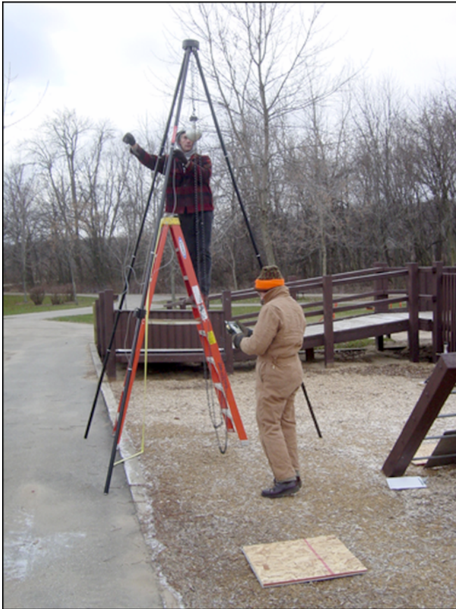
Figure 13—Impact testing on beach path was similar to impact test conducted at a playground using a 3.05-m (10-ft) drop-height.
