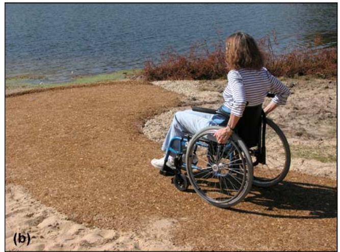
Figure 12—Testing bonded beach path with (a) battery-powered and (b) hand-powered wheelchairs. Shadow near the waterline indicates terminal curb of beach path.
