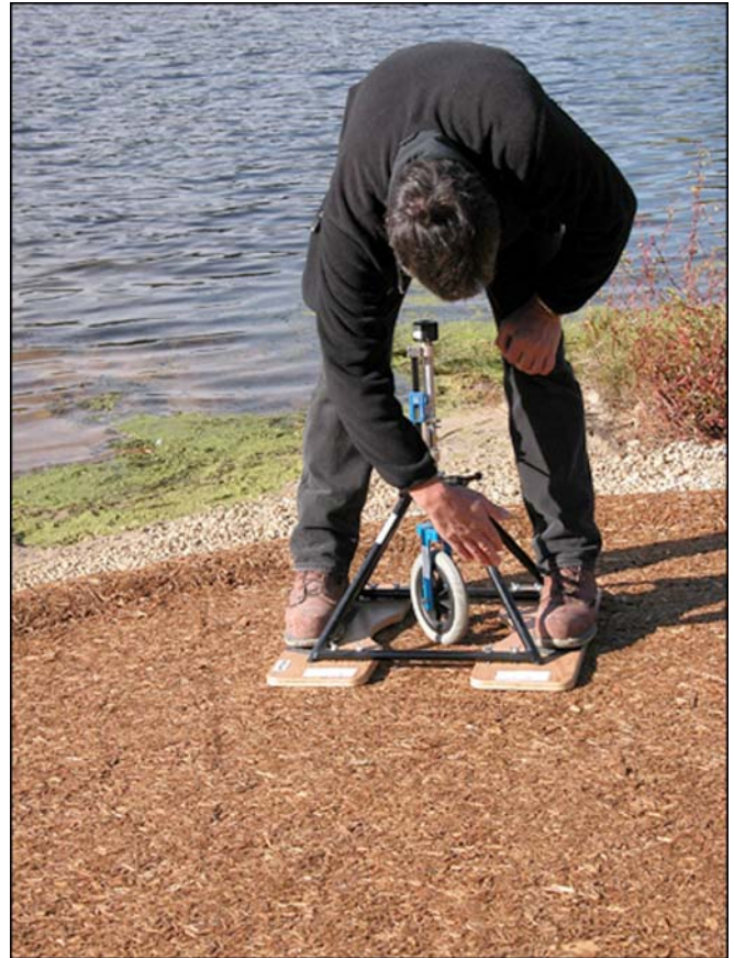
Figure 14—Rotational penetrometer used to measure accessibility.
