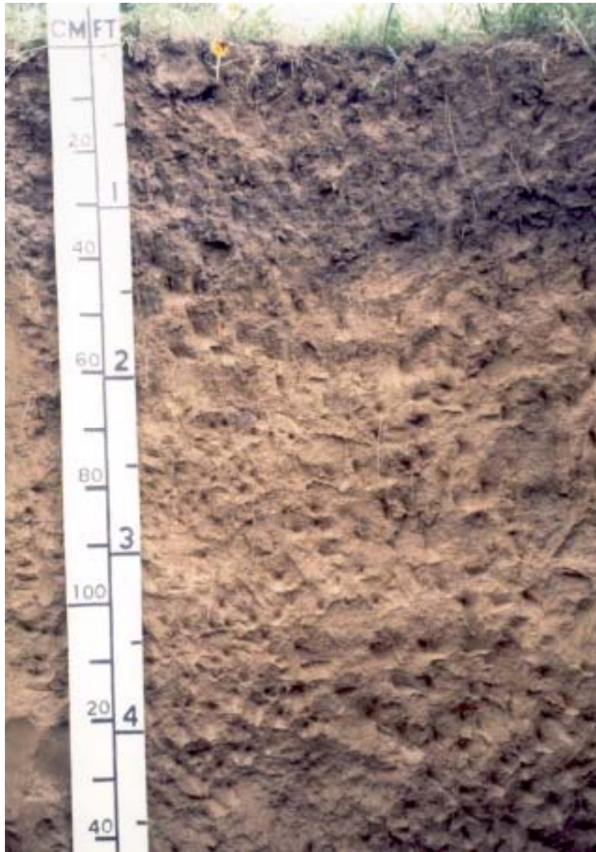
Figure 30.—A profile of Waelder loam, 0 to 1 percent slopes, frequently flooded. Flooding events have deposited loamy and sandy materials.
