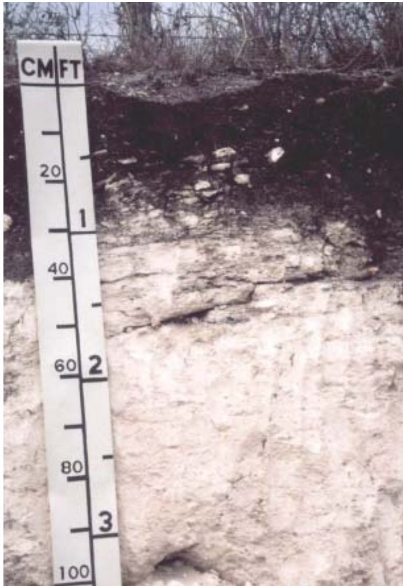
Figure 28.—A profile of Pavelek clay, 0 to 3 percent slopes. The petrocalcic horizon occurs at a depth of 17 inches. Fragments occur in the horizon above the petrocalcic layer.
