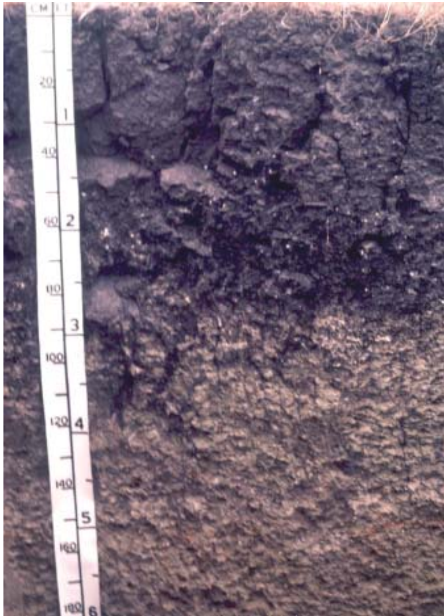
Figure 22.—A profile of Denhawken sandy clay loam in an area of Elmendorf-Denhawken complex, 1 to 3 percent slopes. The clayey texture features include pressure faces and slickensides. Organic matter has stained the surface a dark color.
