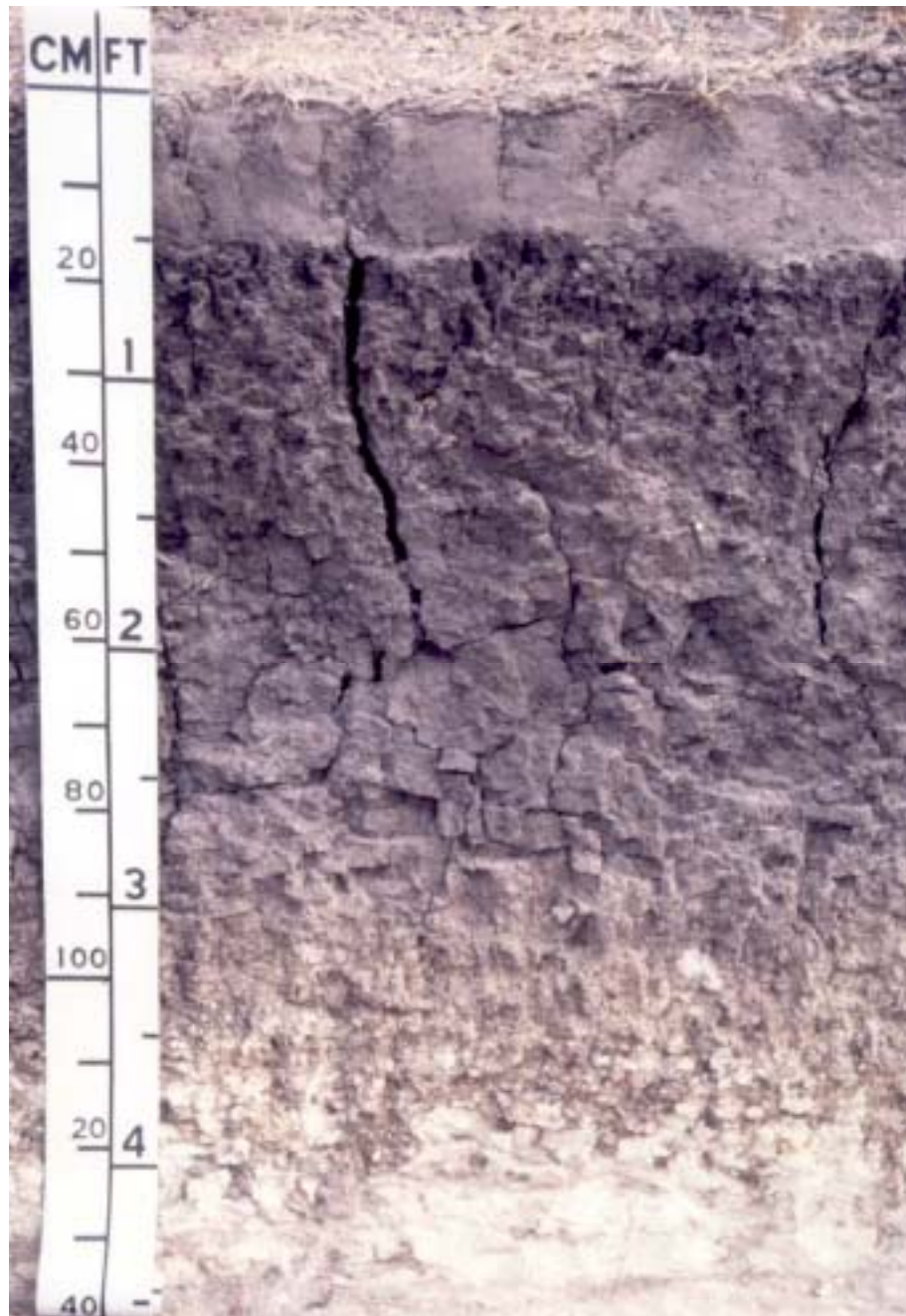
Figure 20.—A profile of Bryde fine sandy loam. The cracks in the subsoil are due to the clayey texture as it dries out. The underlying material, starting at about 55 inches is weakly cemented sandstone.
