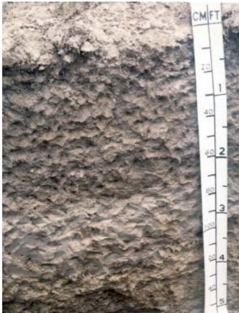
Figure 21.—A profile of Cost loamy fine sand, 0 to 1 percent slopes, occasionally flooded. The subsoil contains a significant amount of sodium which can be toxic to most plants.
