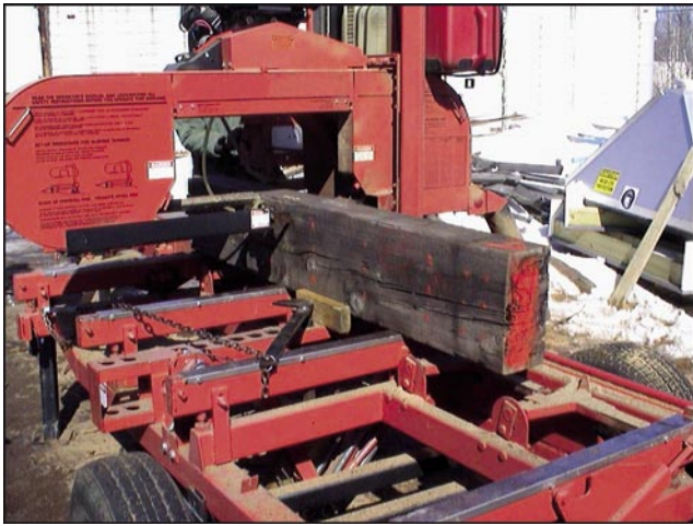
Figure 7—Portable band saw cutting timbers lengthwise along measurement lines.
