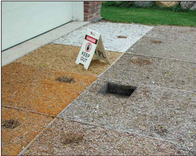
Figure 6—Removal of test sample for determination of density and moisture content of surface layer and EWF beneath surface.
