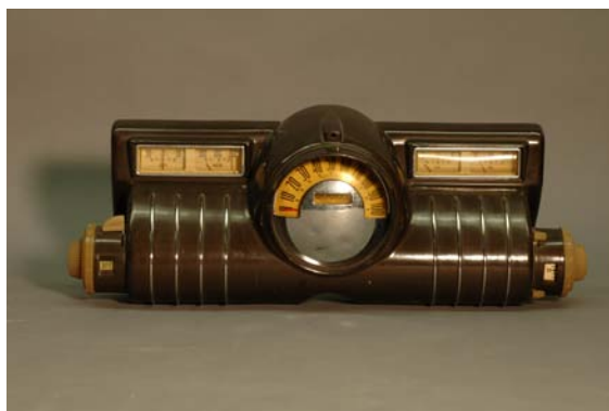
Auto Dashboard, NMAH, 1981.0976.70 Gift of Union Carbide; molded Bakelite with cellulose acetate dials and cellulose acetate covers for speedometer and odometer
