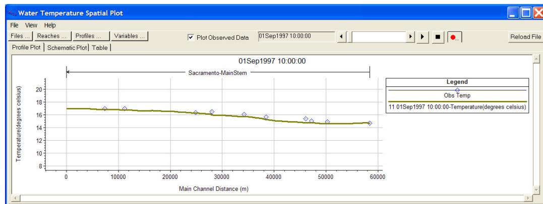
Figure 19-41. Water temperature profile plot showing model simulation and observed data.
