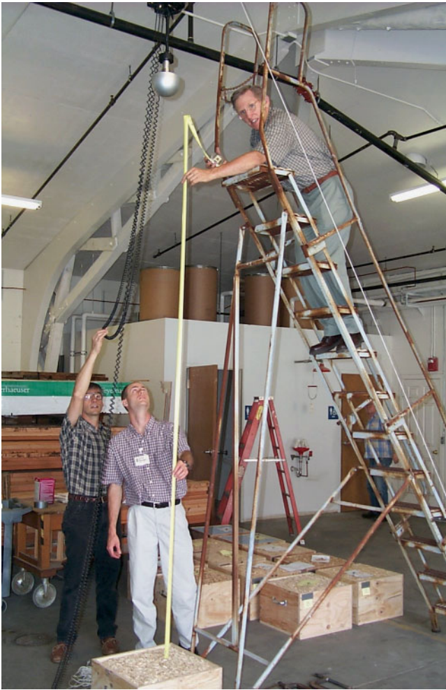
Figure 1—Impact testing set-up for 3-m (10-ft) drop using free-fall test method of ASTM F1292-99.
