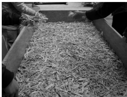
Fig. 22. A view of mat forming for the size of 2000 mm by 1000 mm.
