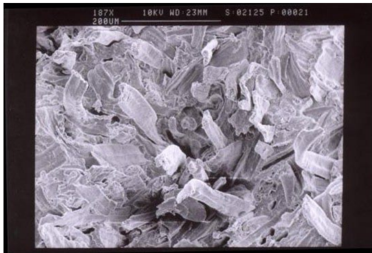
Figure 6. MDF Fibres in Polypropylene Matrix with no Coupling Agent
