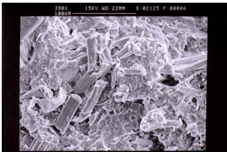
Figure 7. Broken Hemp Fibres In Polypropylene Matrix with no Coupling Agent
