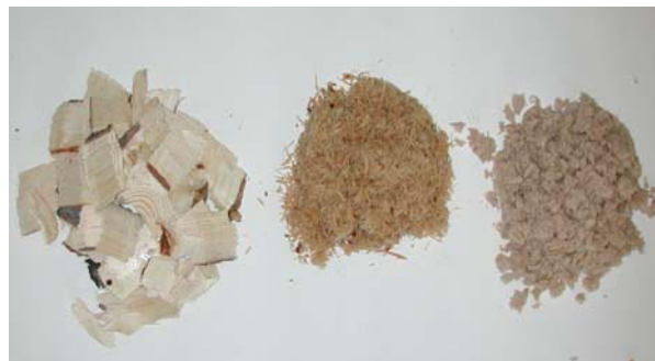
Figure 5. Example of the three processing steps of chips, "tornado" fibers, and refined fiber used when producing 3D engineered fiberboard.
