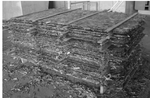
Fig. 24. The boards after pressing were stacked.
