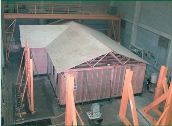
Laboratory test of an irregular one-story house loaded by horizontal forces simulating wind load.
