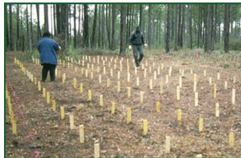
Stake evaluations of the durability of wood used in ground contact.
