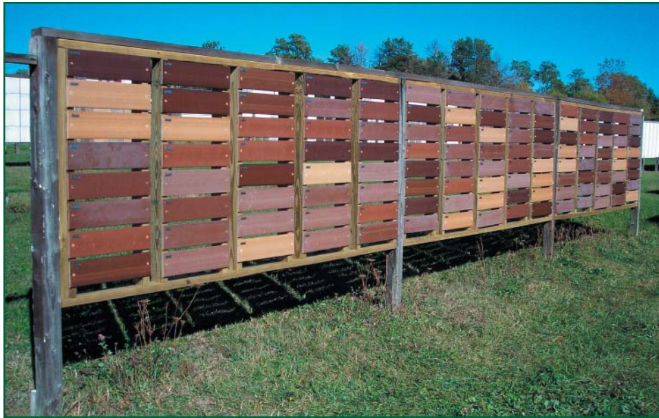
Figure 2. Racks of salt-cedar-, juniper-, and pine-based composites installed in Madison, Wisconsin, to test weathering characteristics.
