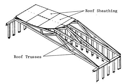
Figure 6 Typical Roof System
