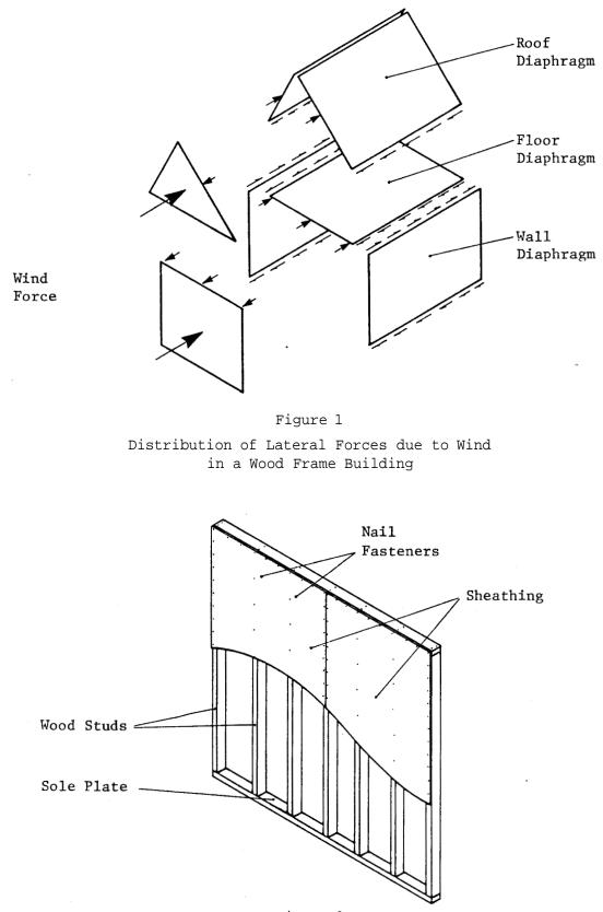
Figure 2 Typical Wall Diaphragm
