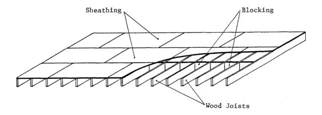
Figure 4 Typical Floor Diaphragm
