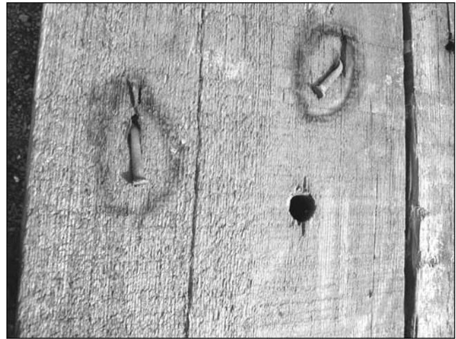
Figure 3—Exposed cut shank nails marked for removal. Also shown is a surface check that may go deep into the lumber piece, affecting potential wood product yield.
