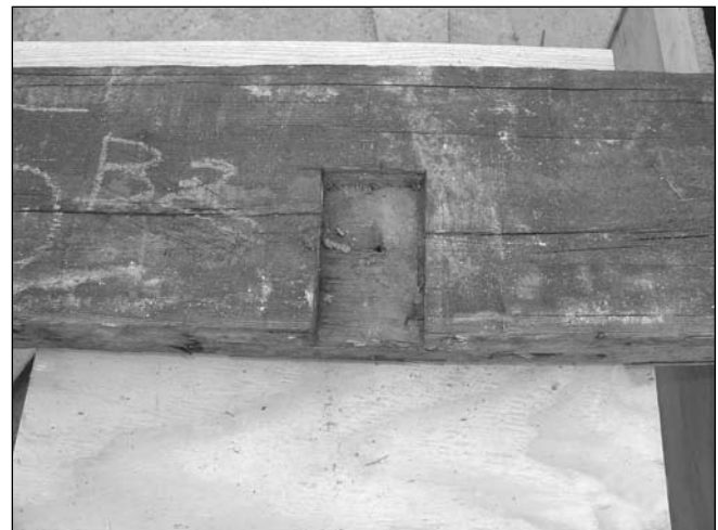
Figure 13—Flaw limiting recovery of a matched pair of feedstock pieces.
