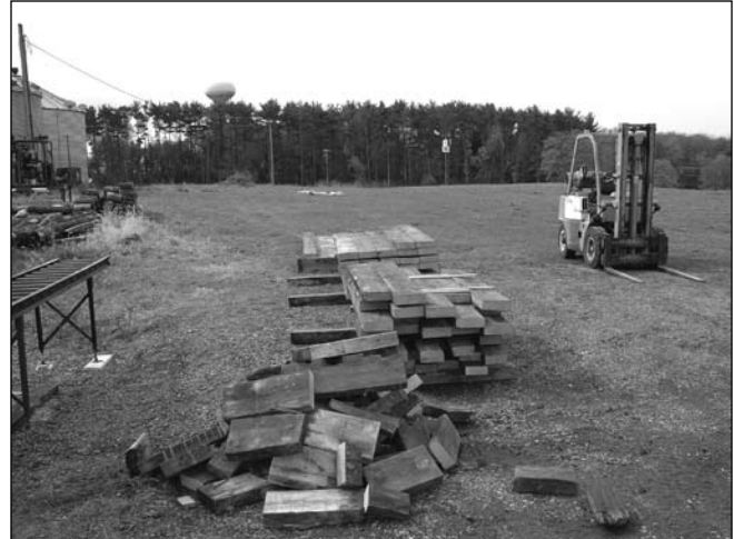
Figure 10—Waste generated through cross-cutting out defect.
