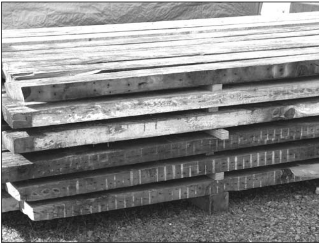
Figure 1—Lumber with stickers placed between the rows and sorted into stacks to allow surface moisture drying.
