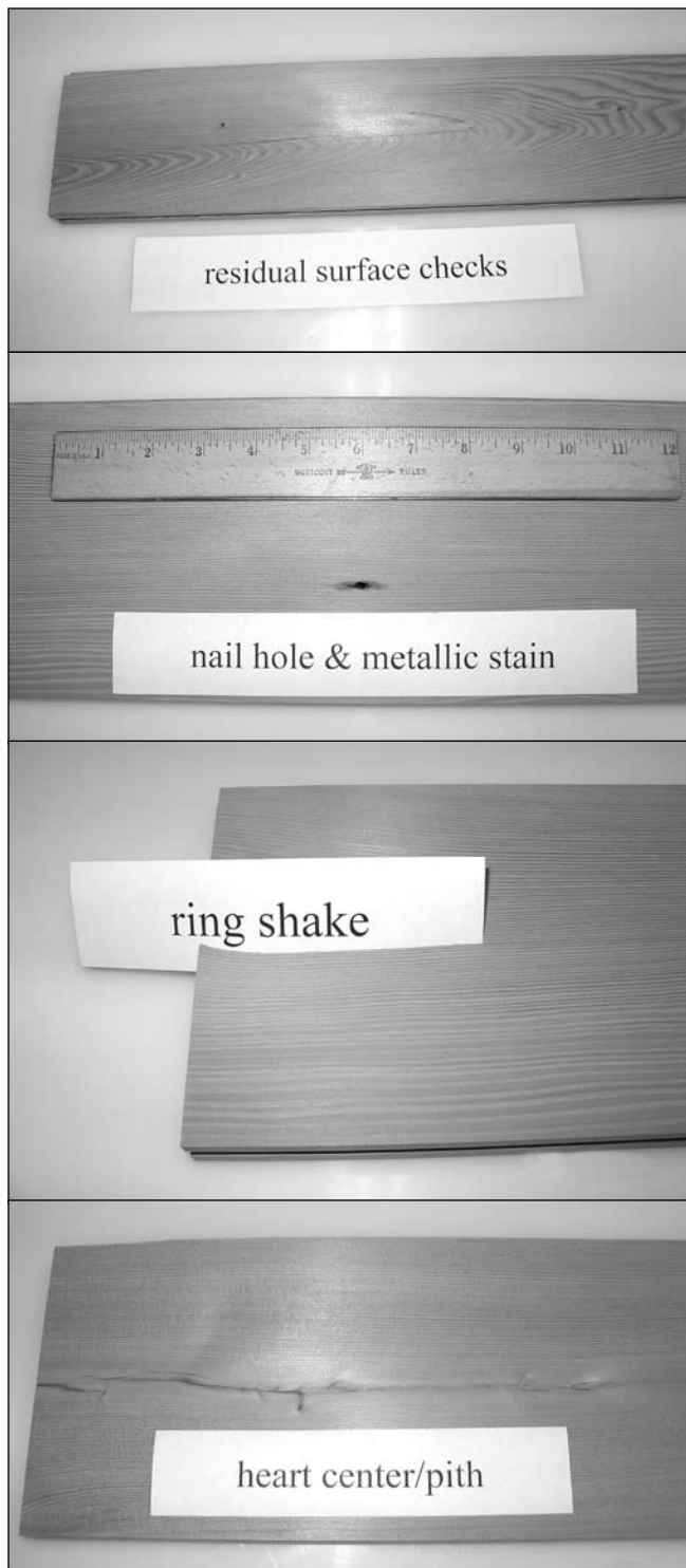
Figure 15—Typical defects found after moulding the lumber. Flooring pattern shown.
