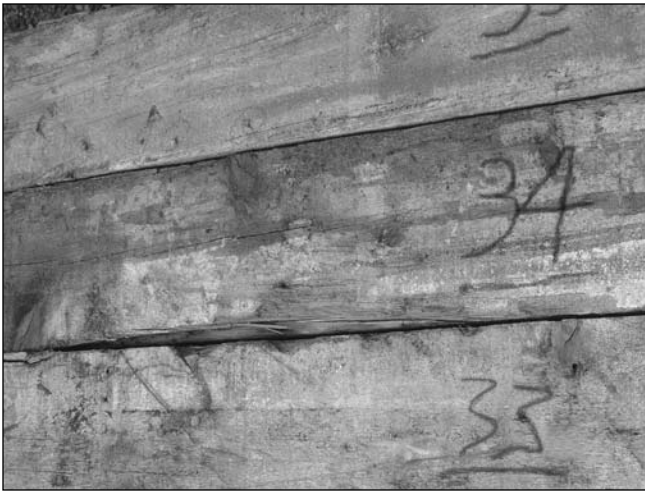
Figure 7—An identification number for each piece was used to track material yields.
