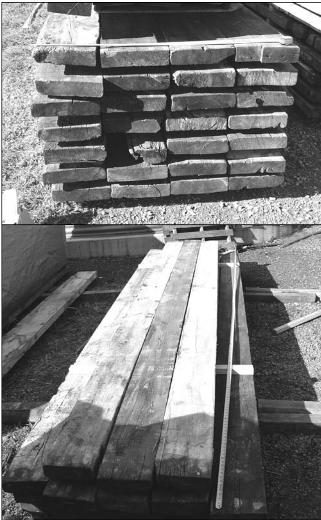
Figure 8—Measurement of lumber width (top) and length (bottom).
