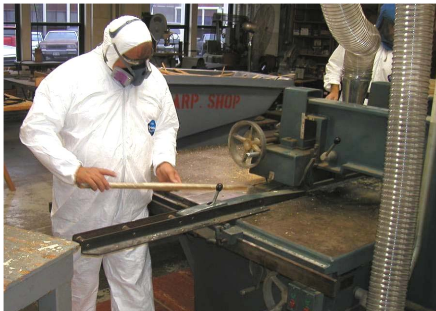
Figure 17. Ripping of siding to width.
