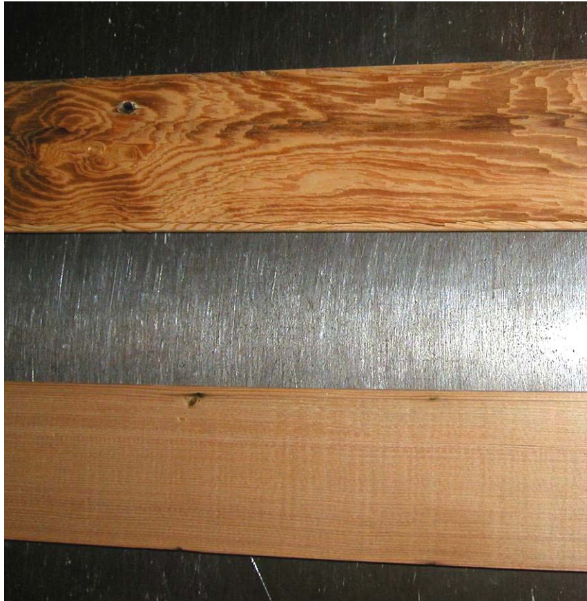
Figure 36. Degradation of wood surface quality (top) due to dulling of HSS knives.
