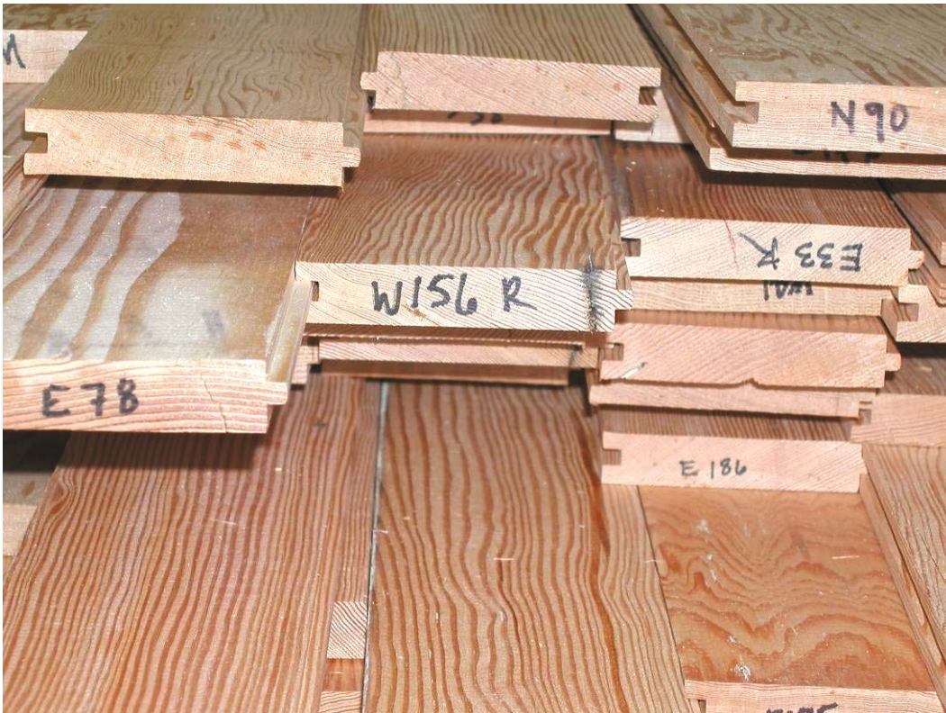
Figure 30. T&G flooring produced from Fort Ord siding.
