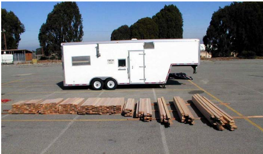
Figure 20. Salvaged Fort Ord wood siding remilled into 5/8 x 4 in. boards for molding into value-added wood products.
