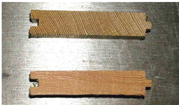
Figure 34. Samples of vertical grain (top) and flat grain (bottom).
