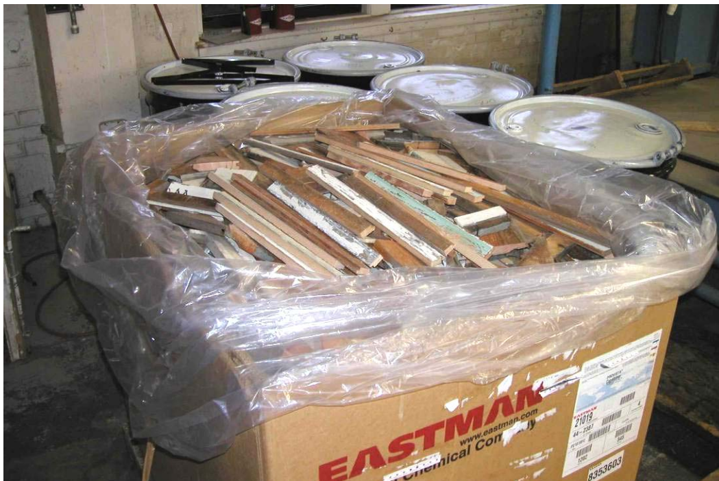
Figure 24. Containers used for storage and shipping of lead-contaminated wood waste.
