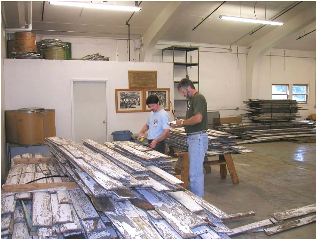
Figure 7. Quantitative inspection of Fort Campbell siding.
