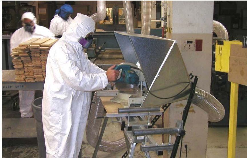
Figure 16. End-trimming with sliding compound miter saw.
