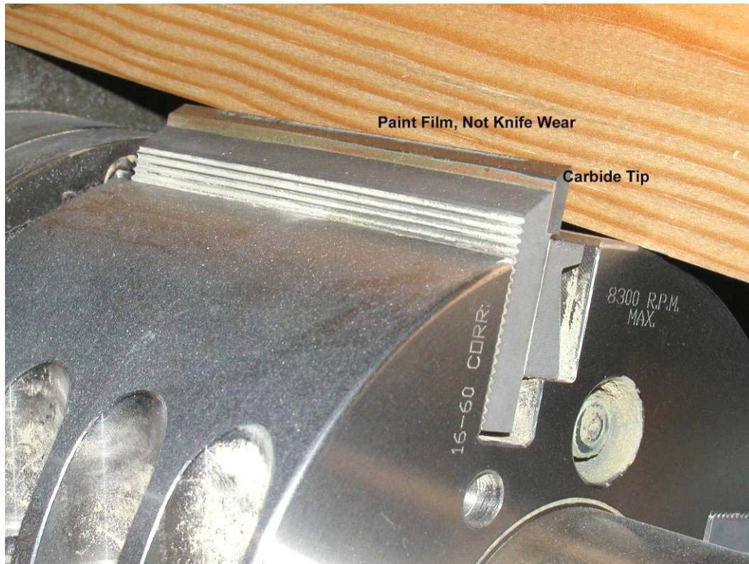
Figure 37. Carbide knife after machining, showing sharp edge with traces of paint residue.
