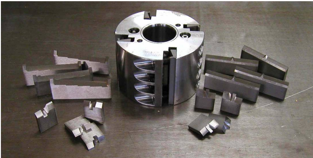
Figure 13. High-speed steel profile knives and Hydroloc™ cutter head.
