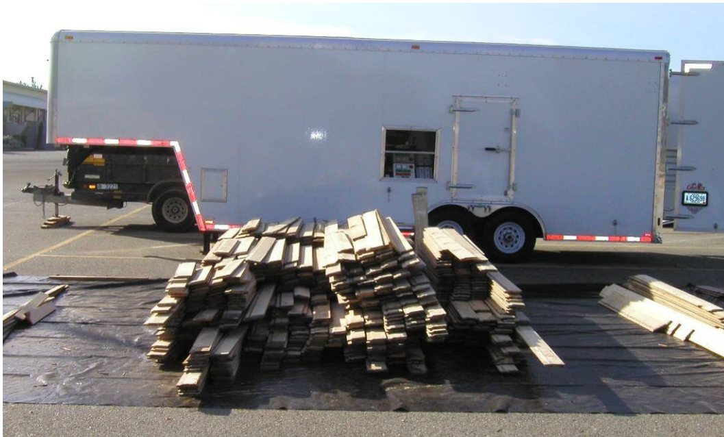
Figure 8. Fort Ord siding provided for remanufacture by Auburn.
