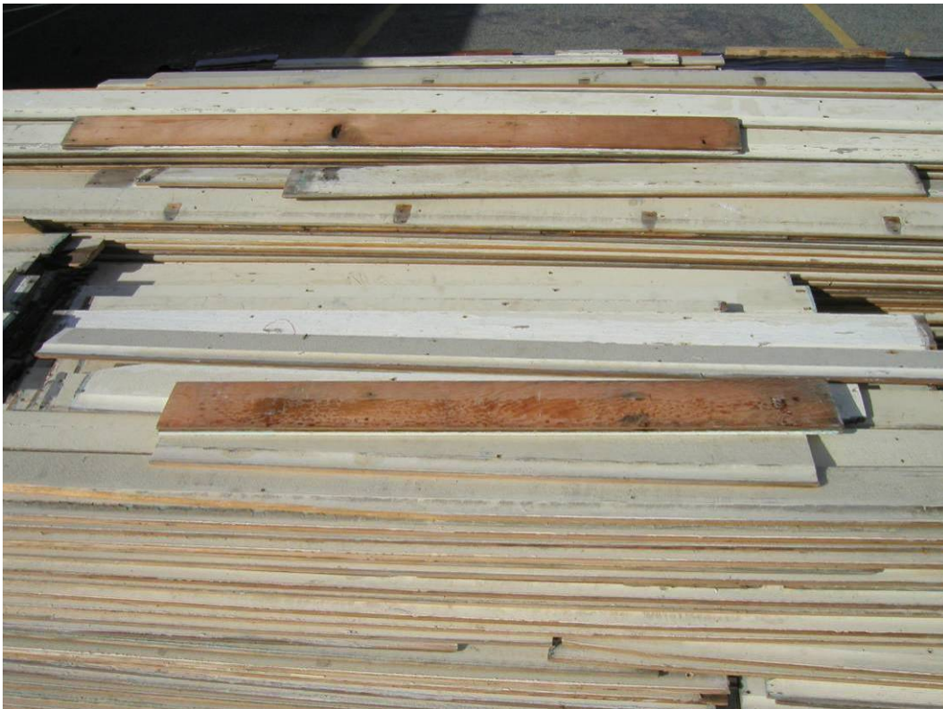
Figure 6. Douglas fir siding salvaged from Fort Ord.
