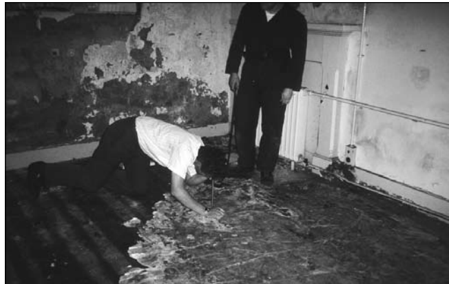
Clausen's early detection test kit can detect decay and stop it before it has a chance to cause irreparable damage to wood.
