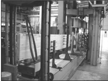
Glulam beam test.
