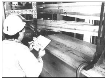
Mapping of failure propagations in glulam beams.
