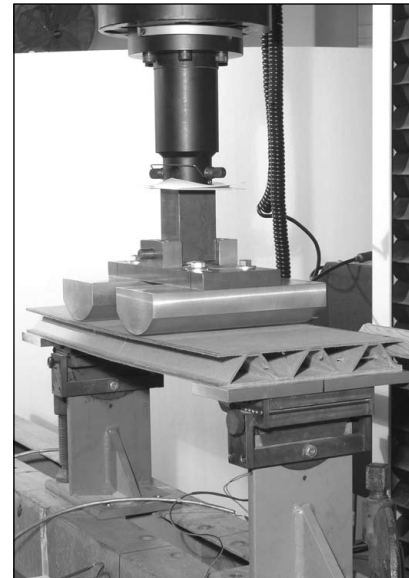
Third point strength bending test on corrugated fiberboard.
