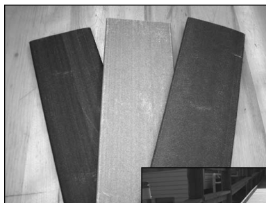
Wood-plastic composite boards made of saltcedar (left), pine (center), and juniper (right). The decking to the right is made of wood-plastic composite boards.
