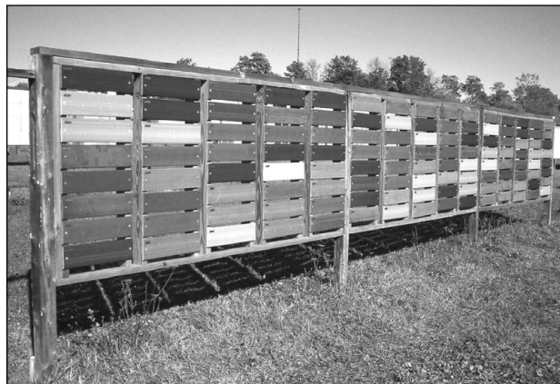
Wood-plastic composite boards on a test rack for natural weathering.
