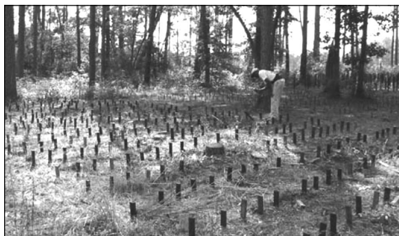
Field stake testing is extremely important when evaluating new wood treatments.
