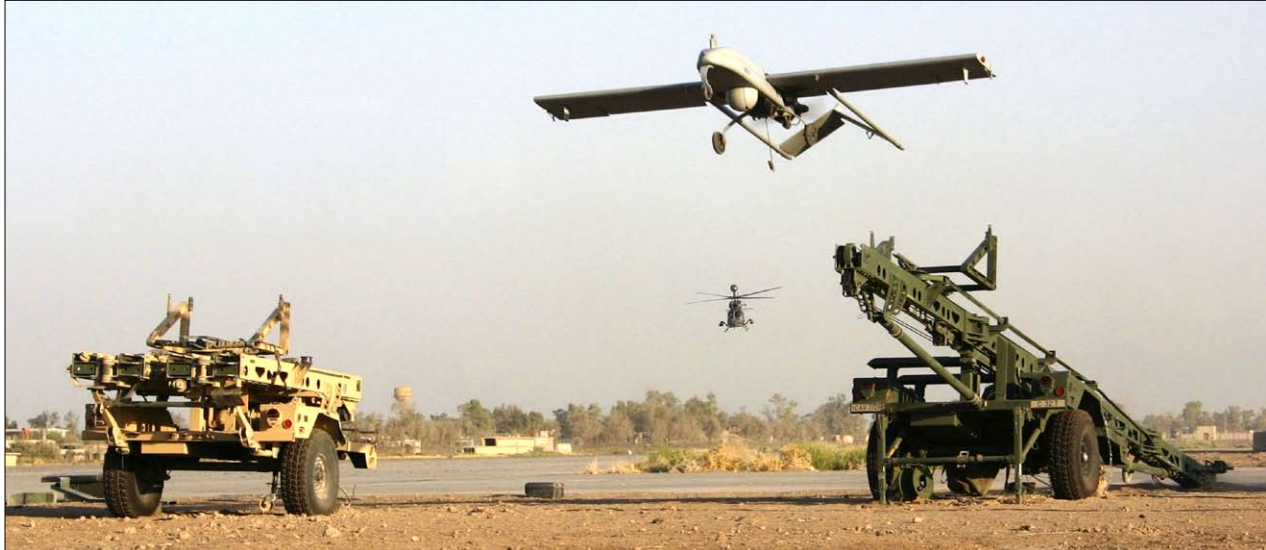
A propeller-driven Shadow 200 unmanned reconnaissance vehicle is launched at a base in Iraq. (Photo courtesy of AAI Corporation)
