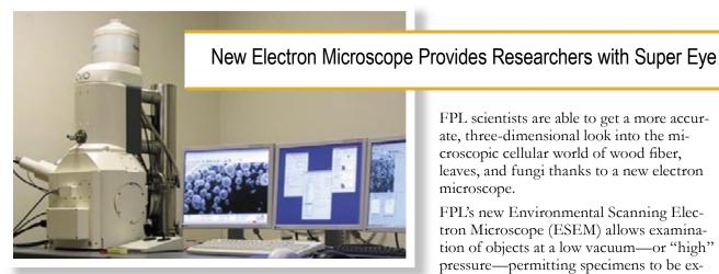
FPL's new electron microscope can reveal threedimensional surface texture of biological specimens without the distortion caused by sample-preparation measures required by older instruments.
