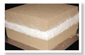
FPL's compositeresearch team examines the engineering performance of chicken-feather and wood fiber composites in a variety of configurations. Shown here, prior to being pressed into medium density fiberboard, is "sandwich" of chicken-feather fiber between two layers of aspen fiber.
