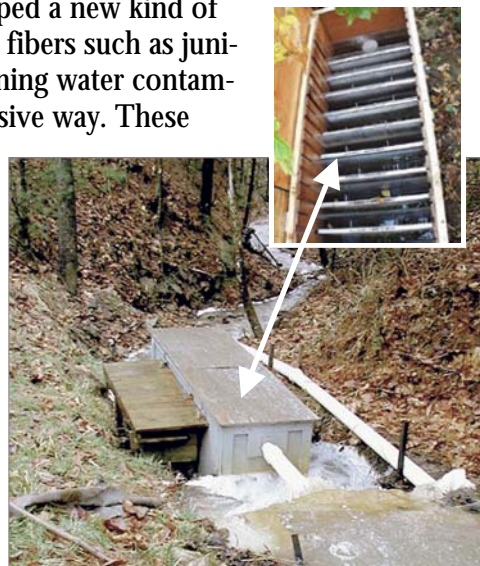
Water filter system showing the wood fiber mats inside.
