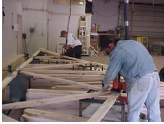
Workers at Kymala Truss in Duluth, MN, assemble a Red Maple truss.
