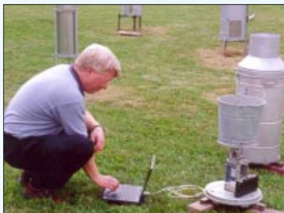
Mark Belding calibrates a new digital recording rain gauge that will be used in the Cook County Network. This network measures rainfall for Lake Michigan diversion accounting for the U.S. Army Corps of Engineers.
