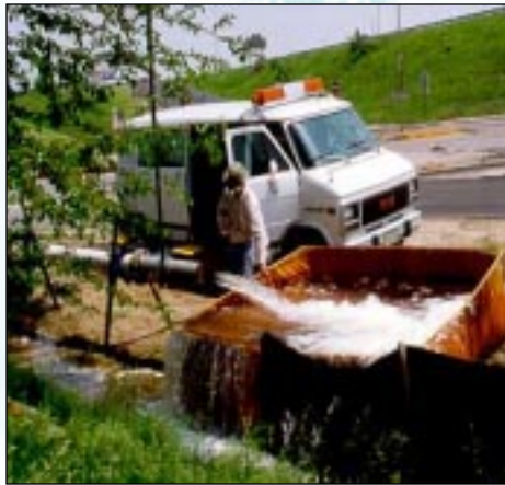
Researchers collect water samples during a step test on IDOT's 25th Street dewatering well.
