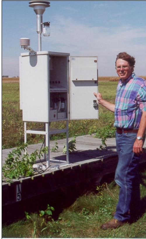
*Clyde Sweet prepares to install a filter in the PM-2.5 sampler at Bondville.*
