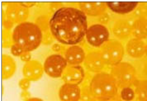
Ion exchange resin removed from a water softener shows signs of iron fouling (dark color) and osmotic cracking.
