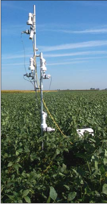
Infrared and thermocouple sensors on a weather tower measure temperatures within and above a crop canopy of soybeans for comparisons to sensors at the same levels over sod at an adjacent ICN site. Also being measured for similar comparisons is the soil moisture at various depths underground.
