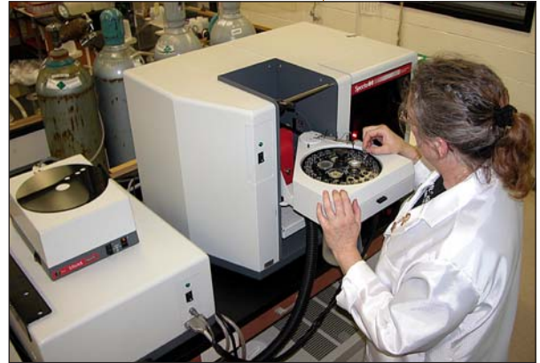
Ruth Ann Nichols prepares PSL samples for arsenic analysis using a graphite furnace atomic absorption spectrometer.
