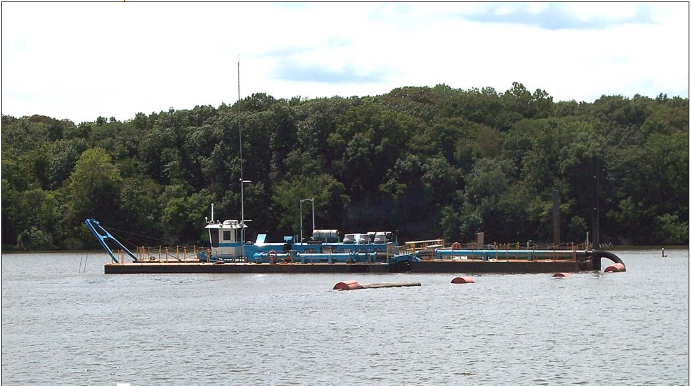
City of Decatur-owned 154-foot dredging equipment removes sediment on Lake Decatur. Photo courtesy of City of Decatur staff.
