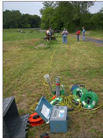
Hydrologists log groundwater levels during an aquifer test at Paris, Illinois.
