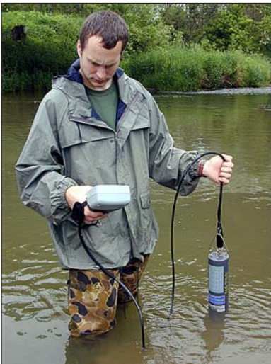
Josh Stevens uses a YSI 6600 data sonde to measure water quality in Court Creek in the Spoon River watershed. The data sonde can be left in the water to provide measurements every 10 minutes over a 2-week period.
