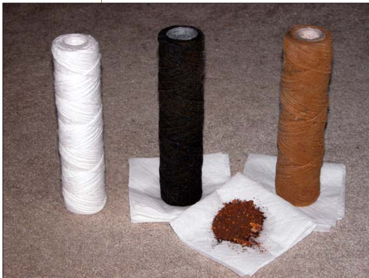
This photo shows a clean water filter (far left) and two others that contain sediment or iron from private wells. The PSL can help solve those problems.
