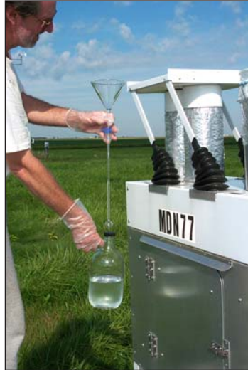
Each week Mike Snider removes the sample from the wet deposition collector attached to the raingage at this monitoring station, which is just one of MDN's 90 sites nationwide.
