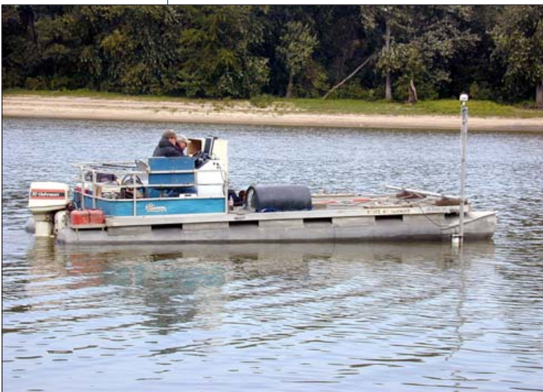
Using an Acoustic Doppler Profiler, Kip Stevenson and Ted Snider collect discharge measurements on the Illinois River near Kingston Mines, Illinois.
