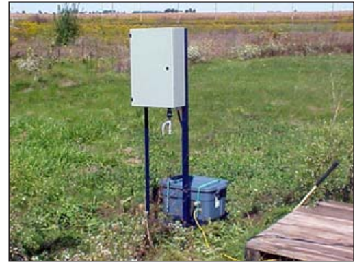
This instrument at Bondville, Illinois, and others from Oklahoma to Ohio measure air samples for gas and particulates, especially ammonia.
