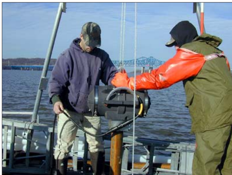
Using a vibrocore, Kip Stevenson and Jim Slowikowski collect sediment samples up to 3 meters long from Peoria Lake.
