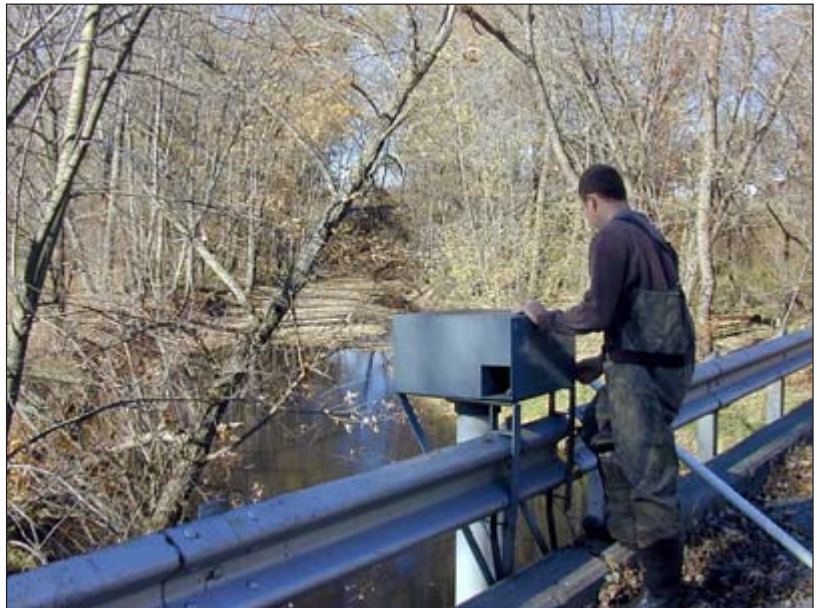
Josh Stevens measures water levels at Long Creek for the Lake Decatur watershed project.
