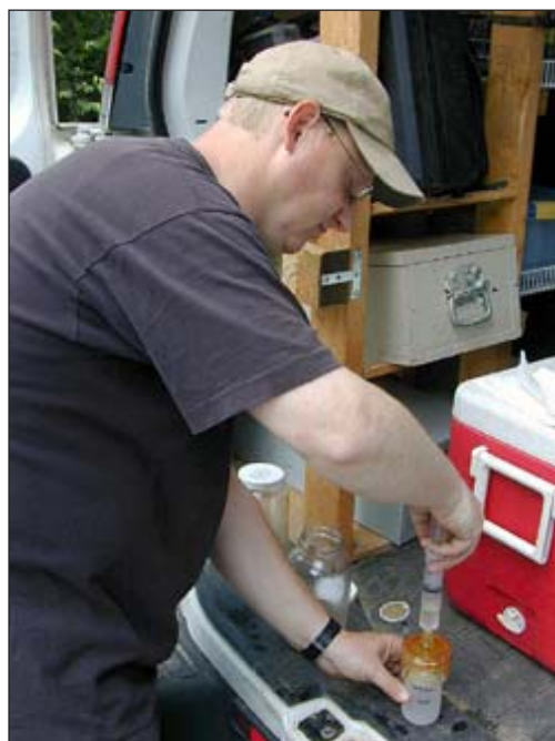
Ted Snider filters a sample from the Sangamon River at Mahomet for nutrient analysis.
