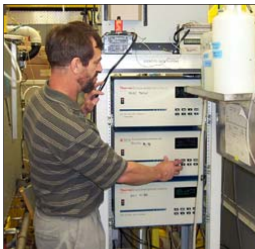
Scientist Allen Williams monitors instruments for analysis of ambient nitrous oxides (NO x ).
