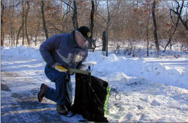
Bill Bogner recovers survey points and determines GPS coordinates.
