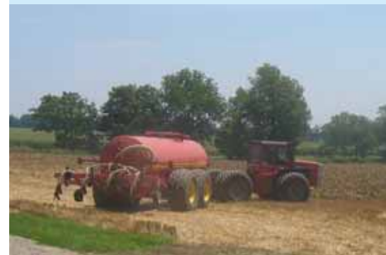
Liquid waste being injected into a field in southern Michigan
