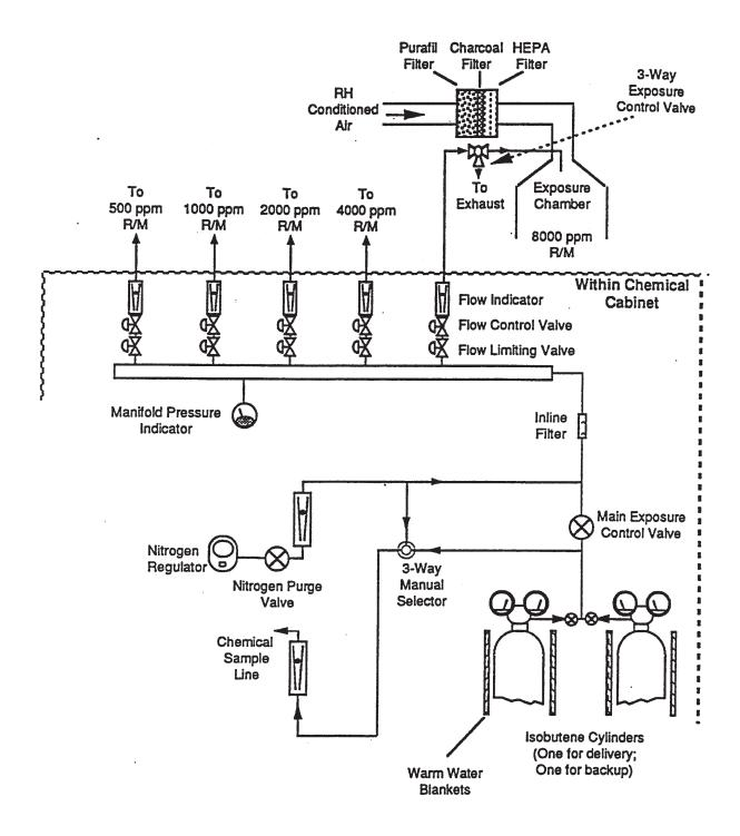
FIGURE J3 Schematic of Generation and Delivery System
