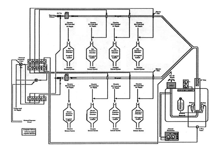
FIGURE F2 Schematic of the Aerosol Generation and Delivery System
