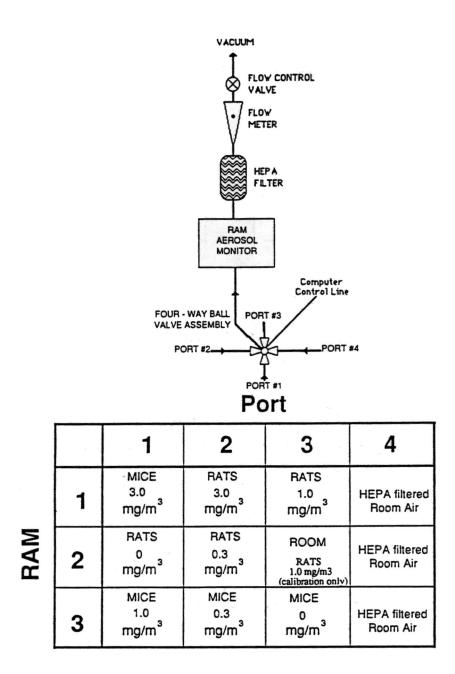
FIGURE F5 Schematic of the Concentration Monitoring System
