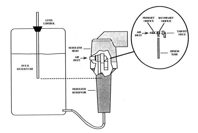
FIGURE F3 Schematic of the RETEC Compressed-Air-Driven Nebulizer
