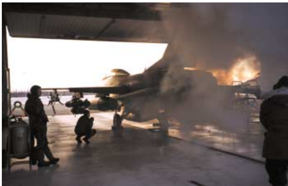
Flight test. Studies of PAH concentrations in aircraft exhaust provide critical information about points during flight-related and ground-support activities—such as engine start-up (above)—when workers may face acute exposures to the possibly carcinogenic compounds.
