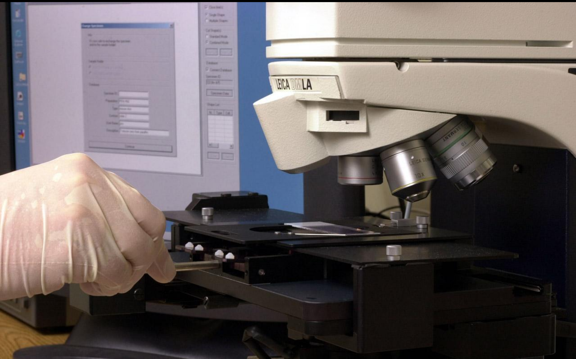
Tube carrier is loaded underneath microscope stage for automation.
