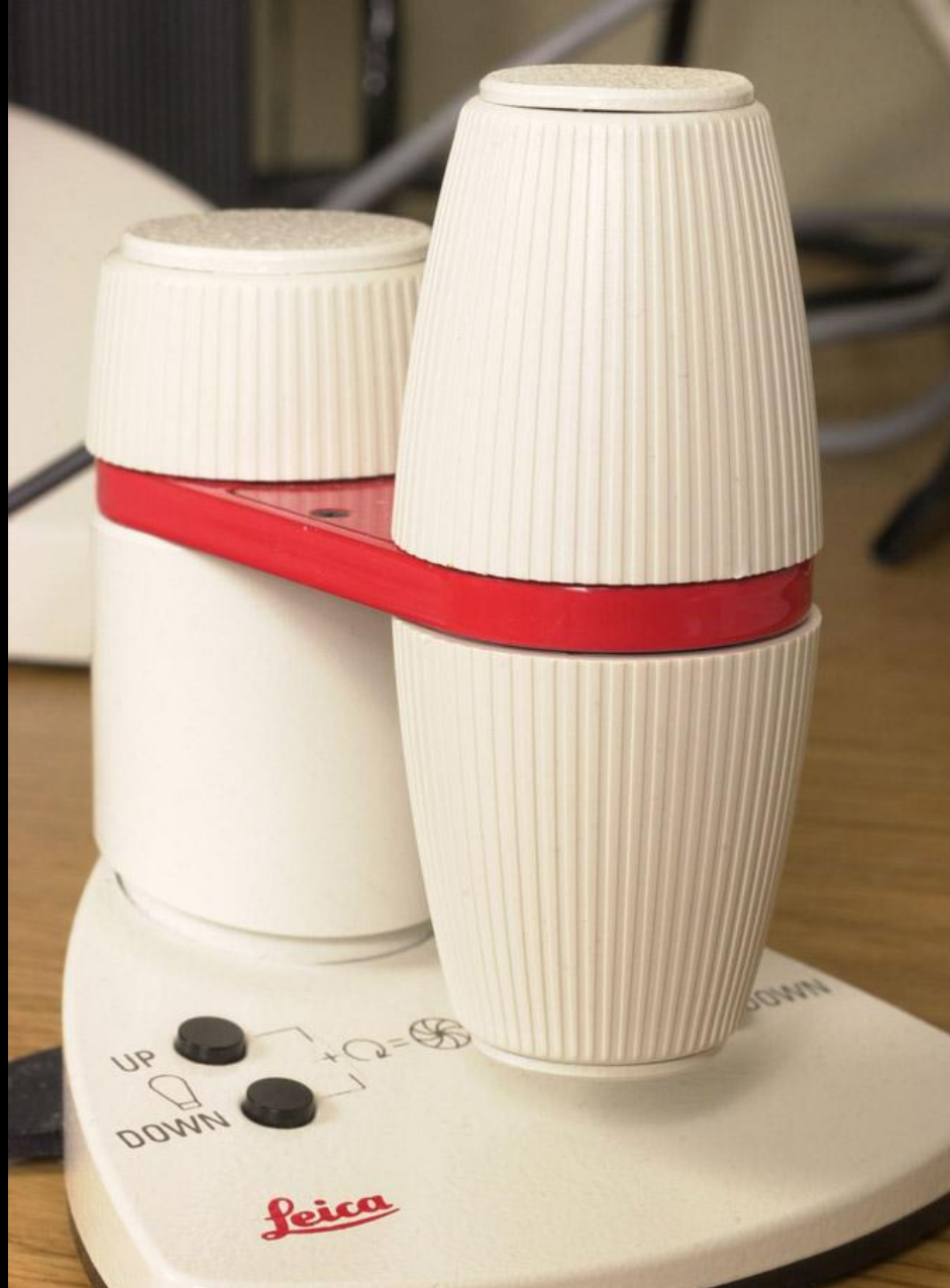
Fully automated controller to guide microscope objectives, stage and lights.
