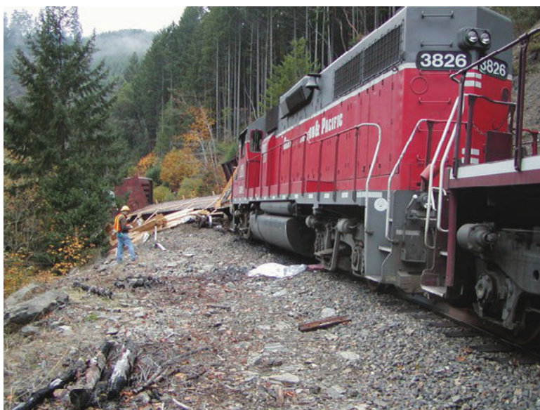
Locomotive with breached diesel tank.
