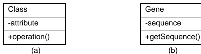
Figure A.3 (a) Schematic for a UML class (b) A simple class called Gene
