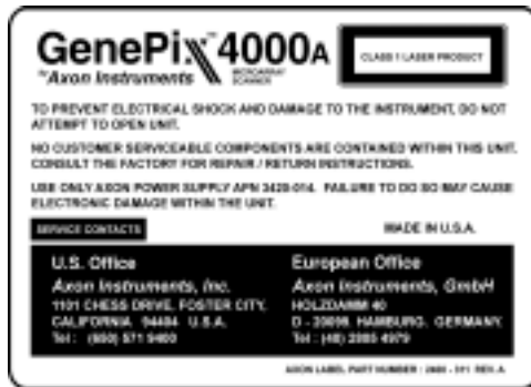
Figure 1. Service Contacts and Warnings Label Label is affixed at the rear of the GenePix 4000A on the upper half of the protective housing. Actual size.
