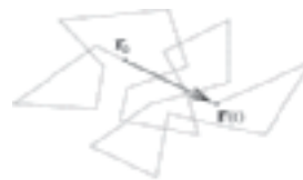
FIGURE 31.2. The Brownian picture of diffusion is best epitomized by this cartoon illustrating a possible path taken by a molecule that is released at point \mathbf{r}_0 at time t = 0 and moves to position \mathbf{r} at a later time t . The molecule undergoes a “drunken walk” whose displacement is characterized by a probability distribution.
