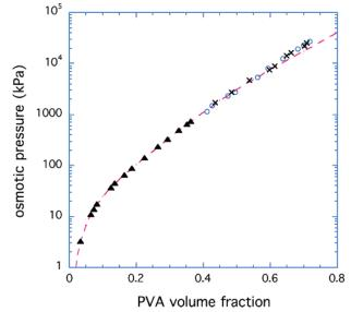
**Figure 4.** Dependence of the osmotic pressure on the volume fraction of the PVA. Open symbols, data measured by the QCM-based osmotic technique; filled triangles, data measured by osmotic deswelling. The dashed curve is the least-squares fit of eq 3 to the data obtained by osmotic deswelling.
