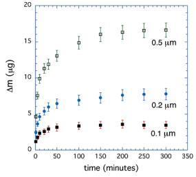
**Figure 1.** Water uptake,  $\Delta m$ , as a function of time for PVA films of different thicknesses. The water vapor pressure was set by a 2% (w/w) NaCl solution.
