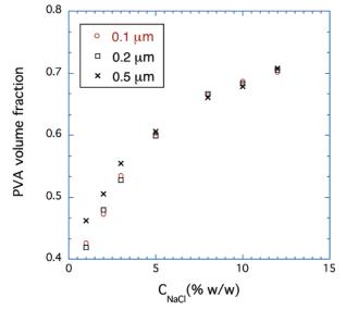
Figure 3. PVA volume fraction as a function of NaCl concentration in the equilibrium bath at 25  $^\circ$ C.
