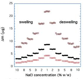
Figure 2. Equilibrium amount of absorbed water,  $\Delta m$ , as a function of NaCl concentration in the equilibrium bath at 25 °C for the PVA samples shown in Figure 1.
