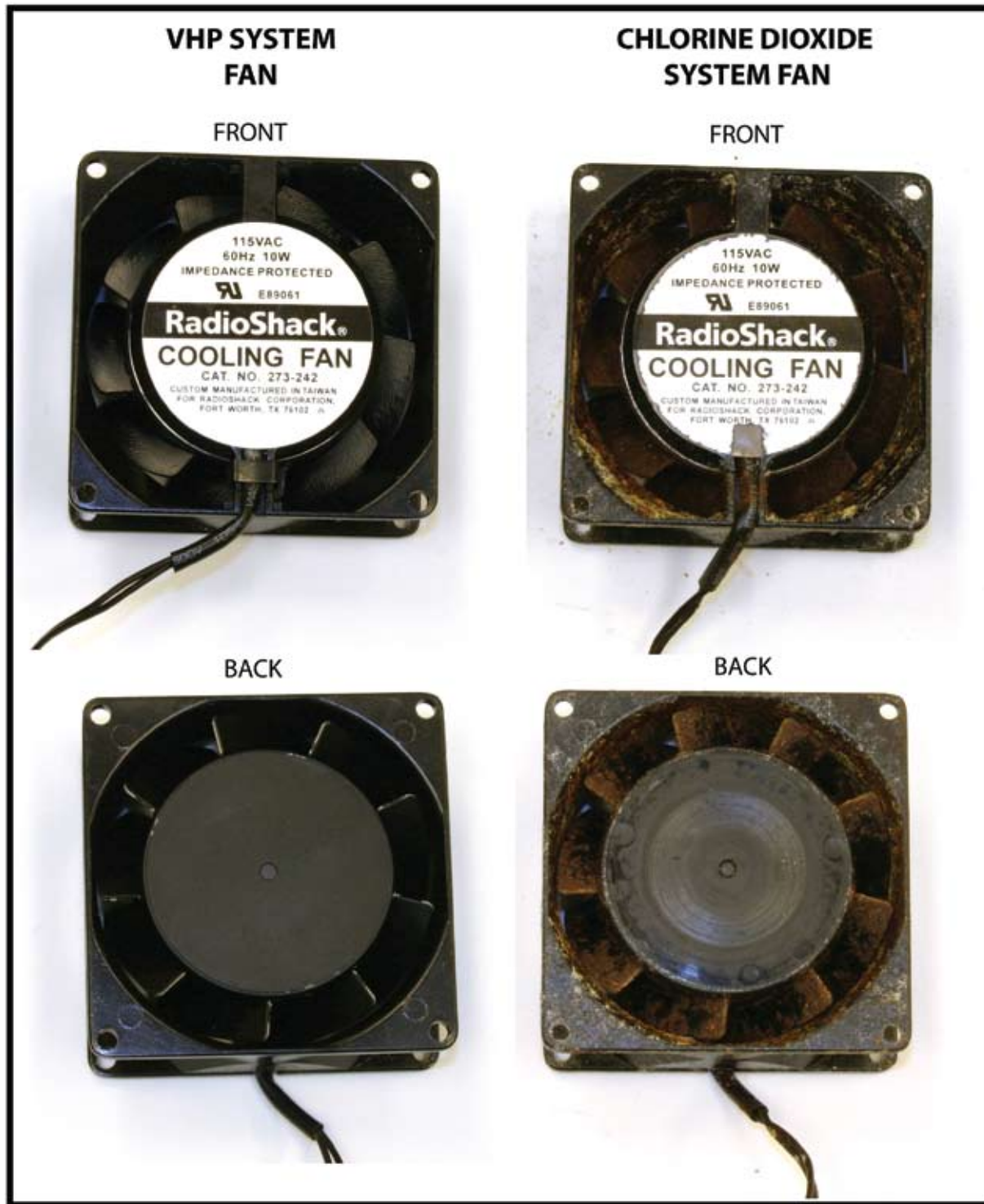
Figure 9. Comparison of Chamber Fans Exposed to Chlorine Dioxide and VHP®.
