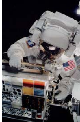
Scientists test polyhedral oligomeric silsesquioxanes (POSS) at International Space Station.
