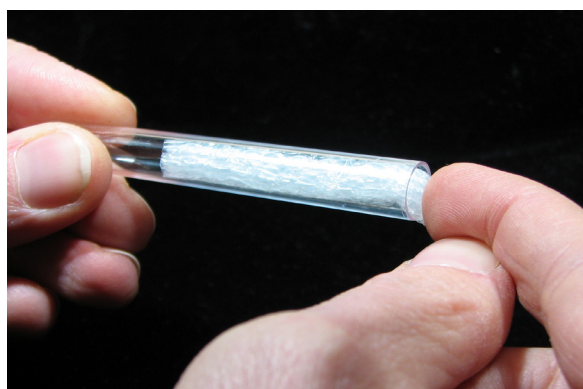
Figure 2. A polyethylene stick in its cuvette demonstrating a firm fit.
