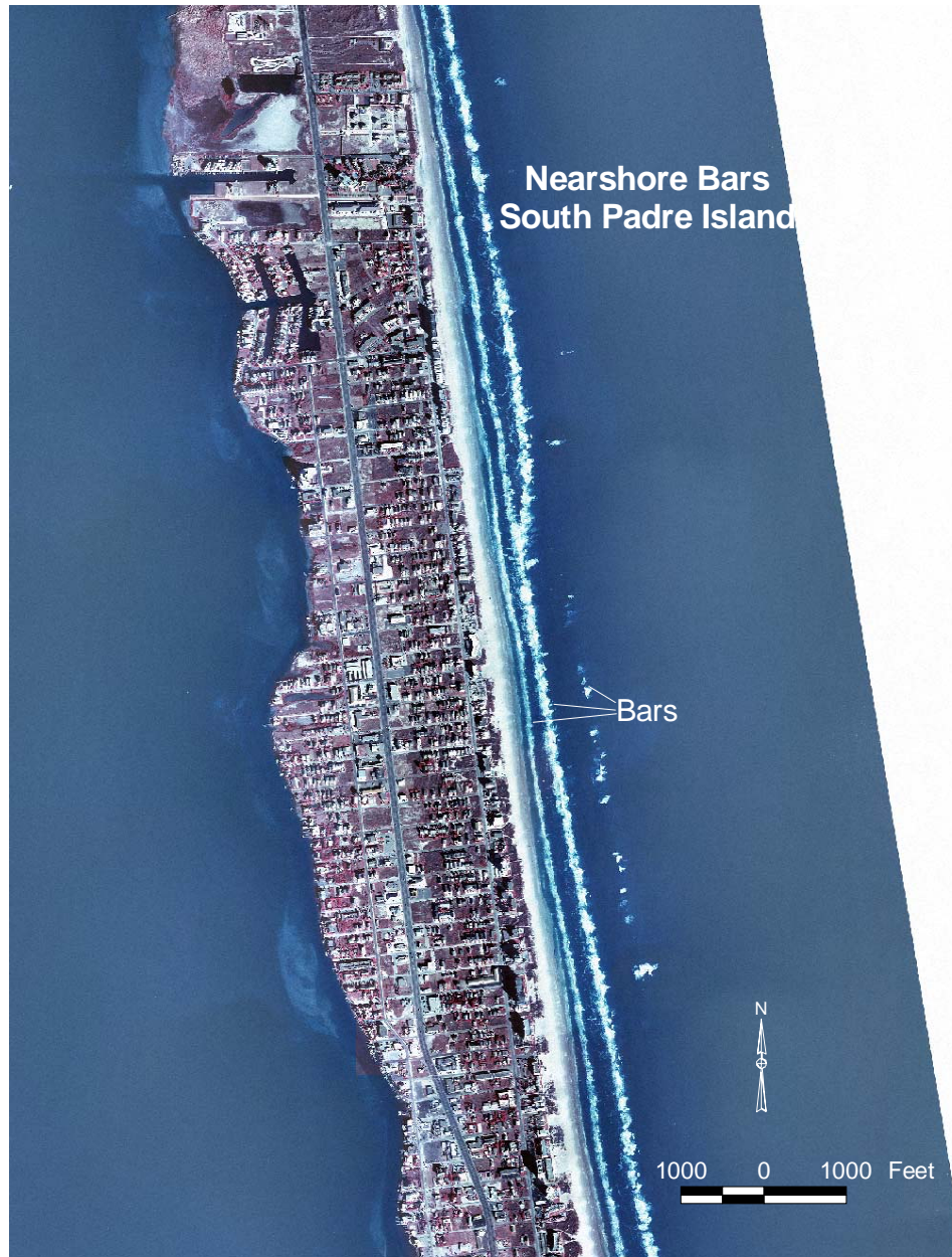
Figure 1. 2002 aerial photograph of South Padre Island about 3.5 miles north of Brazos Santiago Pass. Bars, which store sand, are delineated by breaking waves.
