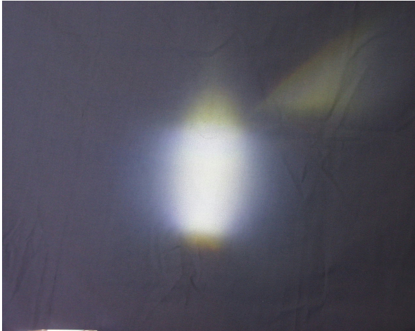
Fig. 2-17 Focal spots of HBO 103 before coarse adjustment
