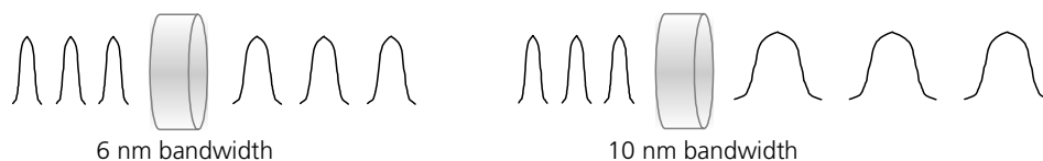
Fig. 10-3 Effect of GVD on short pulses with a broad bandwidth. The broader the bandwidth, the more the pulse is stretched. Longer wavelengths travel faster through the glass than shorter wavelengths in the pulse. Thus, a positively chirped pulse is broadened.
